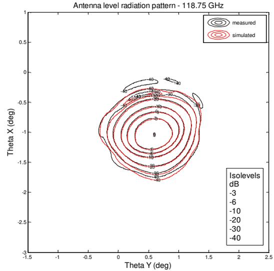
Figure 20. Antenna contour plot – 118.75 GHz – measured/simulated
