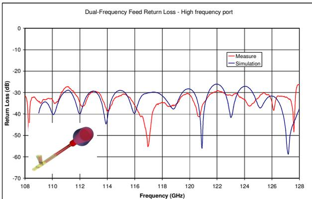
Figure 13. DFF return loss measured/simulated – HF band
