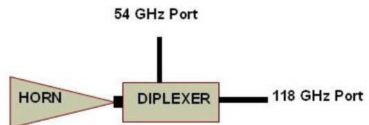
Figure 1. Dual-Frequency Feed (DFF) principle
