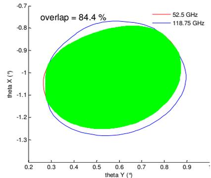
Figure 22. Overlap performance - 52.5 & 118.75 GHz - 3dB contour patterns
