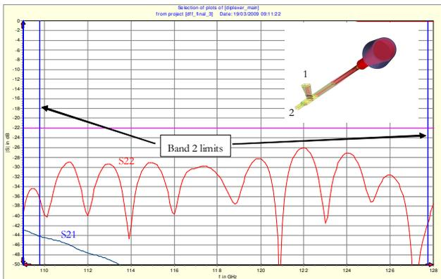
Figure 7. DFF S-parameters 109.75 – 127.75 GHz
