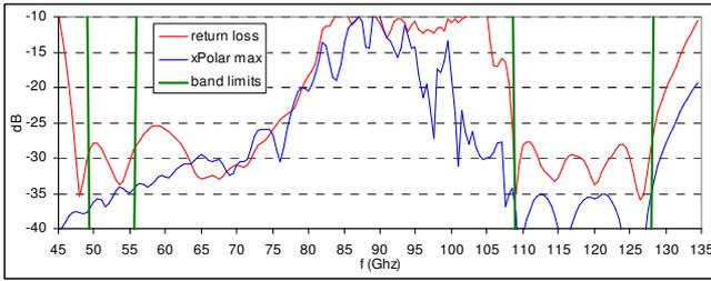
Figure 2. Return loss and cross-polarisation of the horn computed from 45 GHz to 135 GHz
