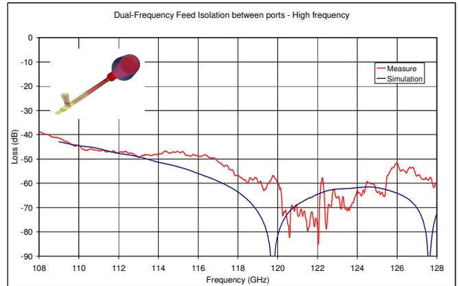
Figure 15. DFF isolation measured/simulated – HF band
