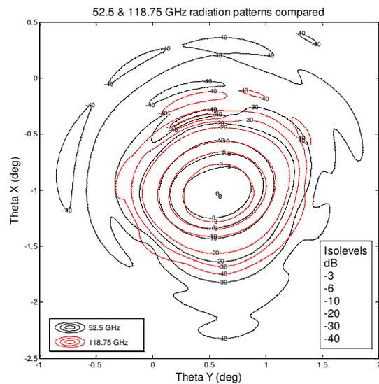
Figure 21. Antenna level contour plot – 52.5 & 118.75 GHz superimposed
