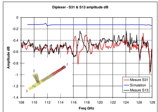
Figure 17. Diplexer insertion loss measured/simulated – HF band
