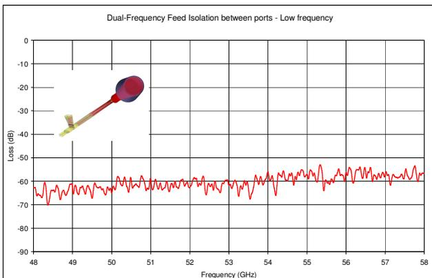
Figure 14. DFF isolation measured/simulated – LF band
