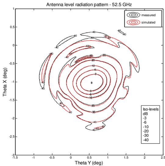
Figure 19. Antenna contour plot – 52.5 GHz – measured/simulated
