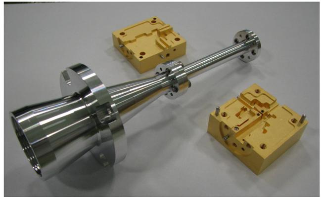
Figure 9. Picture of the horn with the transition and the two half-blocks of the diplexer
