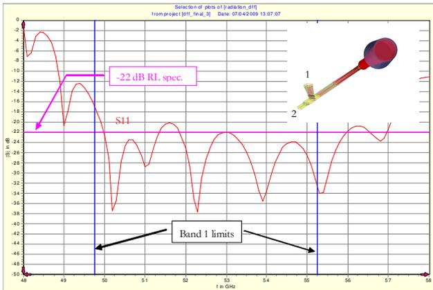
Figure 6. DFF S-parameters 49.75 – 55.25 GHz
