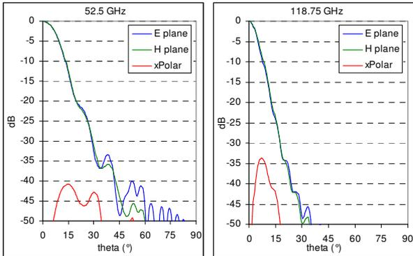
Figure 3. Far field radiation patterns of the horn at centre frequencies
