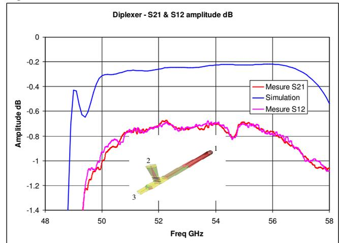
Figure 16. Diplexer insertion loss measured/simulated – LF band
