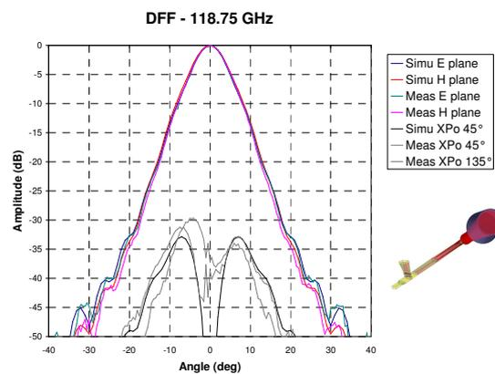
Figure 11. DFF pattern measured/simulated – 118.75 GHz
