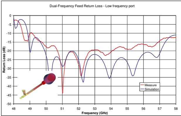
Figure 12. DFF return loss measured/simulated – LF band
