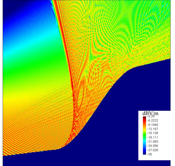
Figure 3: radiation at the end of the valley, calculated using a PO 2D method
