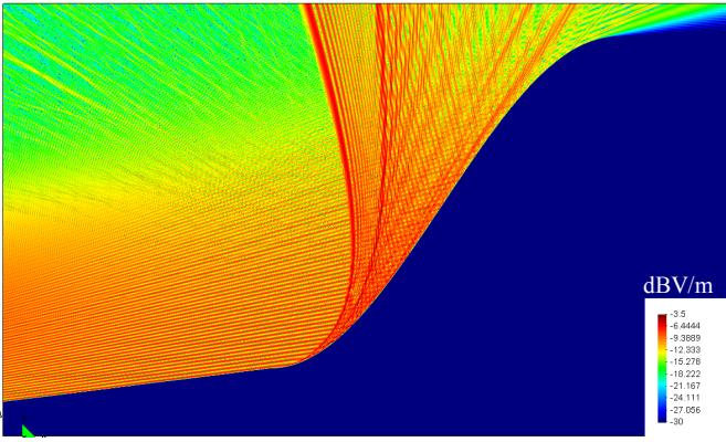
Figure 6: radiation at the end of the valley, calculated using a FDTD 2D method
