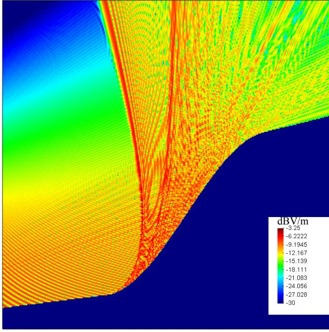
Figure 4: radiation at the end of the valley, calculated using a IPO 2D method
